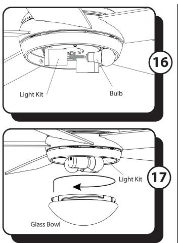
16. Install the E26-base LED bulbs into the sockets of the light kit.
