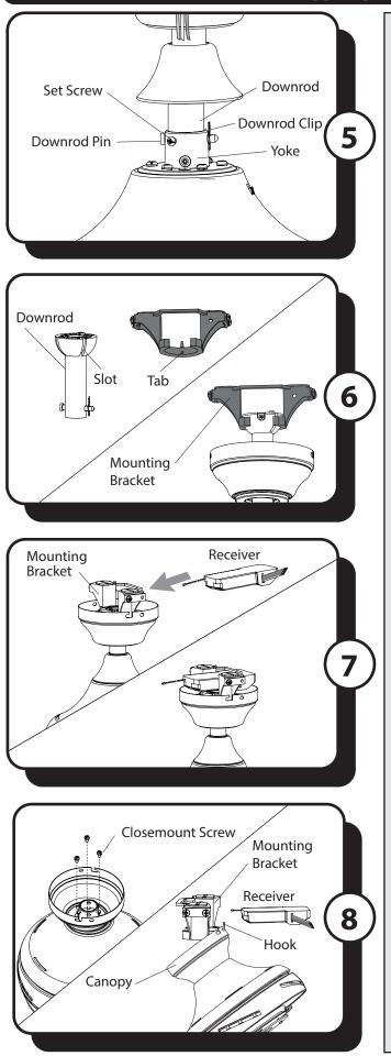
5. Slide the downrod into the yoke of the motor assembly, align the holes, then re-install the downrod pin and downrod clip. Secure with the two set screws and slide the yoke cover down until it rests on top of the motor assembly.
