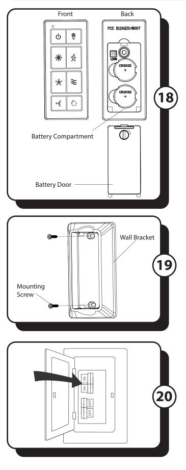
18. Remove the battery door from the back of the remote using a flat-head screwdriver (not included). Insert the two CR2032 batteries into the remote; ensure the positive pole of the batteries face up (as pictured) and then replace the battery door.
