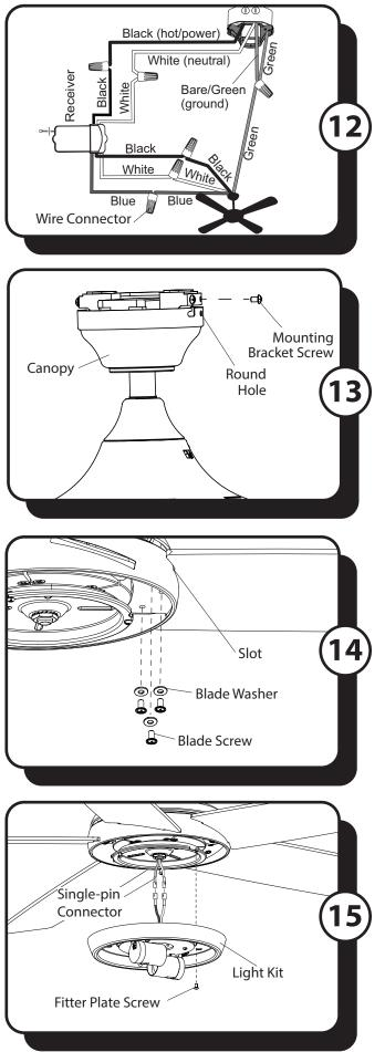
12. Use wire connectors to secure the household supply wires to the receiver and fan according to the wiring diagram and the following instructions:
