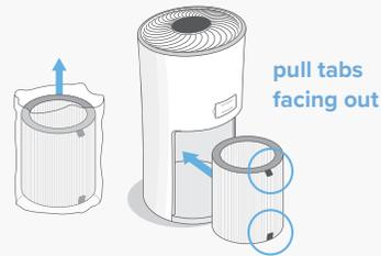
Unwrap the new filter and place it into the housing.
