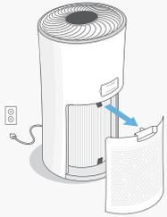
Unplug the air purifier and remove the filter cover.
