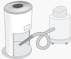
Clean any remaining dust or hair inside the air purifier using a vacuum hose. **Do not** use water or liquids to clean the air purifier.
