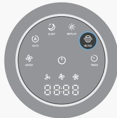
Turn on the air purifier. Press and hold
