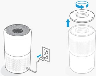
Unplug the air purifier and remove the filter cover.
