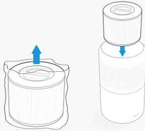
Unwrap the new filter and place it into the housing.
