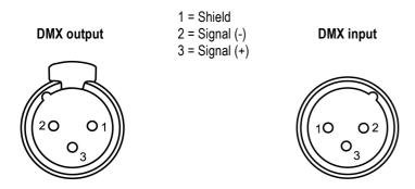
Connect the DMX output of the first unit in a DMX chain with the DMX input of the next unit in the chain. Always connect the the output of one unit with the input of the next unit until all units are connected.
