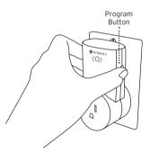
Release program button, press the **ON** or **OFF** button for the desired number on the remote. 4. Pairing is successful when indicator light stops blinking.
