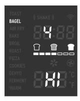
This function crisps the inside of a cut bagel while lightly toasting the outside.
