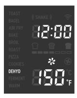
This function combines low and stable heat with automatic airflow to evenly dry out foods without cooking. Ideal for drying fruit or vegetable chips.
