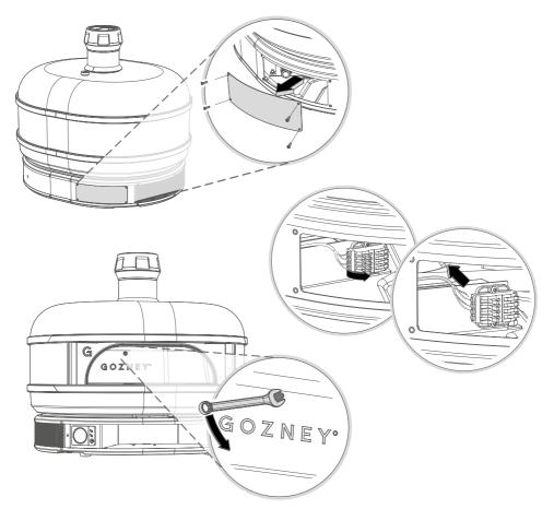
Only when the oven is cold, remove the rear panel to access the probe terminal. The terminal is held with a magnet so can be removed from the dock easily to gain better access. Lift all the levers on the left hand side of the terminal to release the probe wires. Unscrew the probe from inside the oven and pull the old probe out the mouth of the oven.
