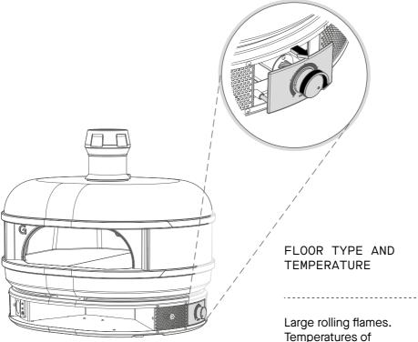
After moving the fire over the mesh puck turn the control dial on the ash tray to the fully open position. This allows more oxygen to get to the fire and will help you achieve a good rolling flame across the top of the oven. Always wear oven gloves when adjusting the dial on the ash tray. Temperatures of 750°F (400°C+)
