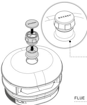
The flue is designed to have a rain guard which has a 1/4" (5mm) gap from the Dome.
