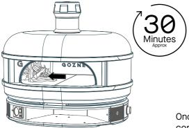
Once the fire has established itself in the center of the oven push it over to the left and continue to feed it for approximately 30 minutes or until the oven is fully saturated.
