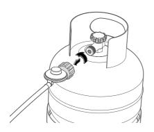
After cooking, be sure to turn off the gas from the gas canister first before turning of Dome. This will allow any gas left in the burner or pipe to be used up safely. Three minutes after turning the gas off it will be safe to remove the regulator and turn the control dial back to the off position.
