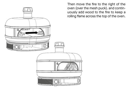
The flame from the wood fire should roll across the length of the oven's roof. Avoid overfeeding the fire, there should never be flames coming out the mouth of the oven. If you are struggling to get a good flame, ensure the wood you are using follows our guidelines at the beginning of this chapter.
