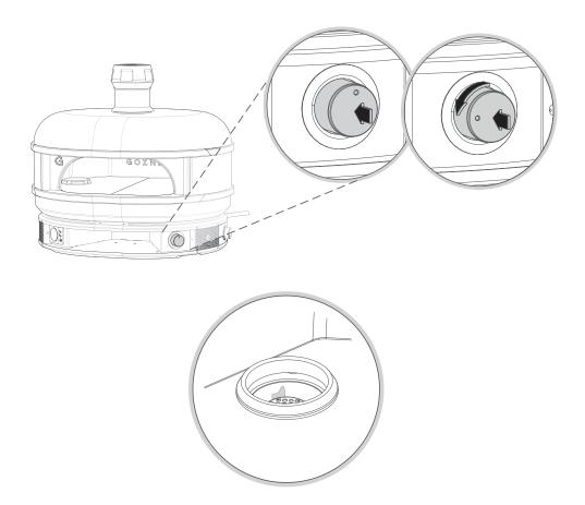
Note on first firing on changing a gas cylinder you may need to push the control knob in for an extended period of time. To allow gas to flow from the bottle to the pilot assembling.
