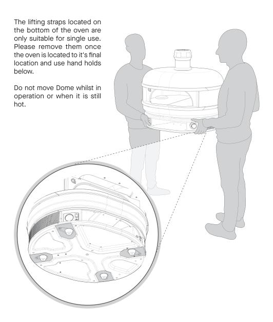
Never attempt to move the oven on your own. Two people should pick up the oven lifting from under the rounded ends of the oven, do not use the mouth of the oven as a lifting point.
