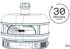
Once the fire has established itself in the center of the oven push it over to the left and continue to feed it for approximately 30 minutes or until the oven is fully saturated.
