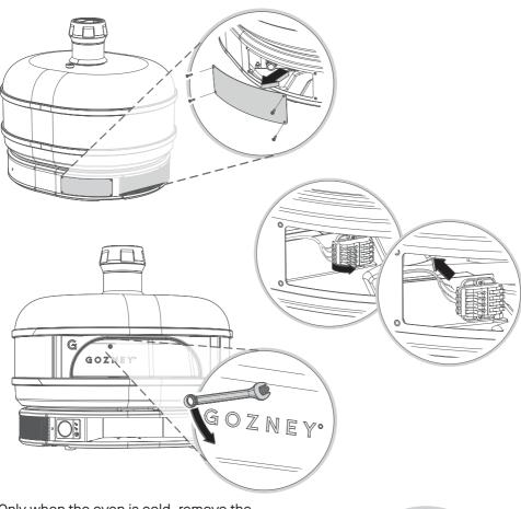
Only when the oven is cold, remove the rear panel to access the probe terminal. The terminal is held with a magnet so can be removed from the dock easily to gain better access. Lift all the levers on the left hand side of the terminal to release the probe wires. Unscrew the probe from inside the oven and pull the old probe out the mouth of the oven.
