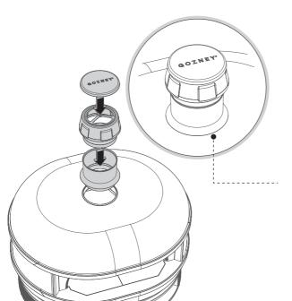
The flue is designed to have a rain guard which has a 1/4" (5mm) gap from the Dome.
