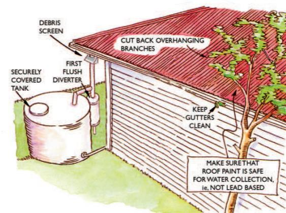
Roof areas should be kept clear of overhanging vegetation to prevent leaves and other debris from falling onto the catchment. Overhanging branches also give rodents, cats, and possums access to the roof and allow birds to roost above it.
