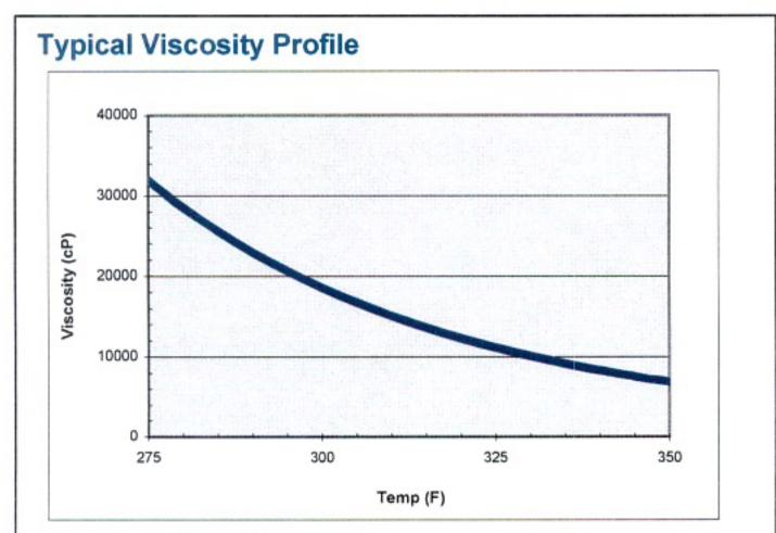
(Data collected using Brookfield viscometer/thermocel using a thermocel load of 10.5g, spindle #27, at 10rpm)
