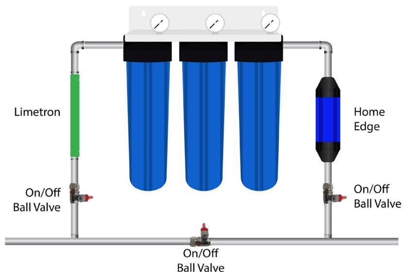
**NOTE:** The 2 x tapered nipples provided with the Home Edge MUST be used to screw into the Home Edge or the warranty will not be covered, Please read instructions & warranty conditions in Home Edge box.
