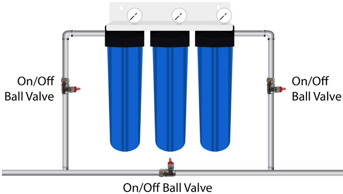
**Diagram 2:** MWF 20" x 4.5" Triple Big Blue Whole House Water Filter System Complete with Hard Water Conditioner
