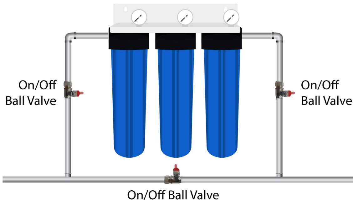
**6.** After complete installation, do not open the valve on the mains yet, fully open an outside tap nearest to the whole house big blue filter system first.
