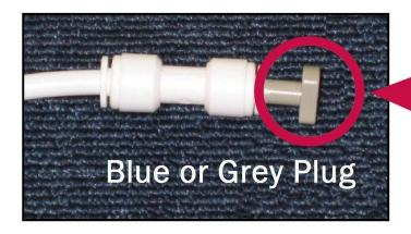
BEORE YOU BEGIN: You must remove the Blue or Grey plug from the drinking water line, or no water will come out. Replace this cap when system is not in use to prevent bacteria in the water line.
