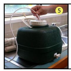
Place filtered water line directly into desired storage container for fresh, Flouride free water. Be sure to leave your storage container on the sink area in case of overflow.
