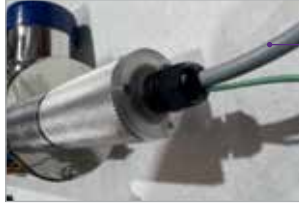
Sealing Nut complete with UV Lamp installed and cable secured
