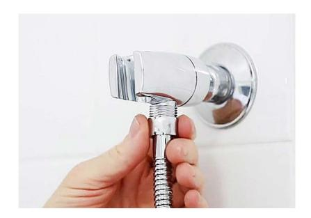
**9.** Remove the protector sticker from the ½" male end thread of the shower filter handle. Connect the remaining shower hose end connector onto the ½" male threaded connector of the shower handle. Make sure it's tight to avoid leaking. However, avoid over tightening, as this might damage the threads of the shower handle.
