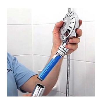
**4.** Get the new cartridge and insert it into the shower handle. The cartridge is reversible and can go in any way. Insert the shower handle back into the showerhead, make sure the slots on the shower handle are in line with the pegs in the shower head. Push gently and twist to the right to lock. For optimum performance, you can reverse the cartridge every 3 months.
