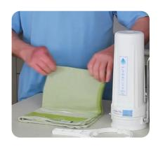
2. Lay the benchtop water filter on its side on the towel. The spout must be facing away from you. This will make it stable and easy to work with. This will also allow you to have more leverage in opening the benchtop water filter housing.
