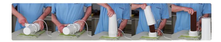
5. Get the new Aragon cartridge, remove any wrapping and insert it into the filter head cap.
