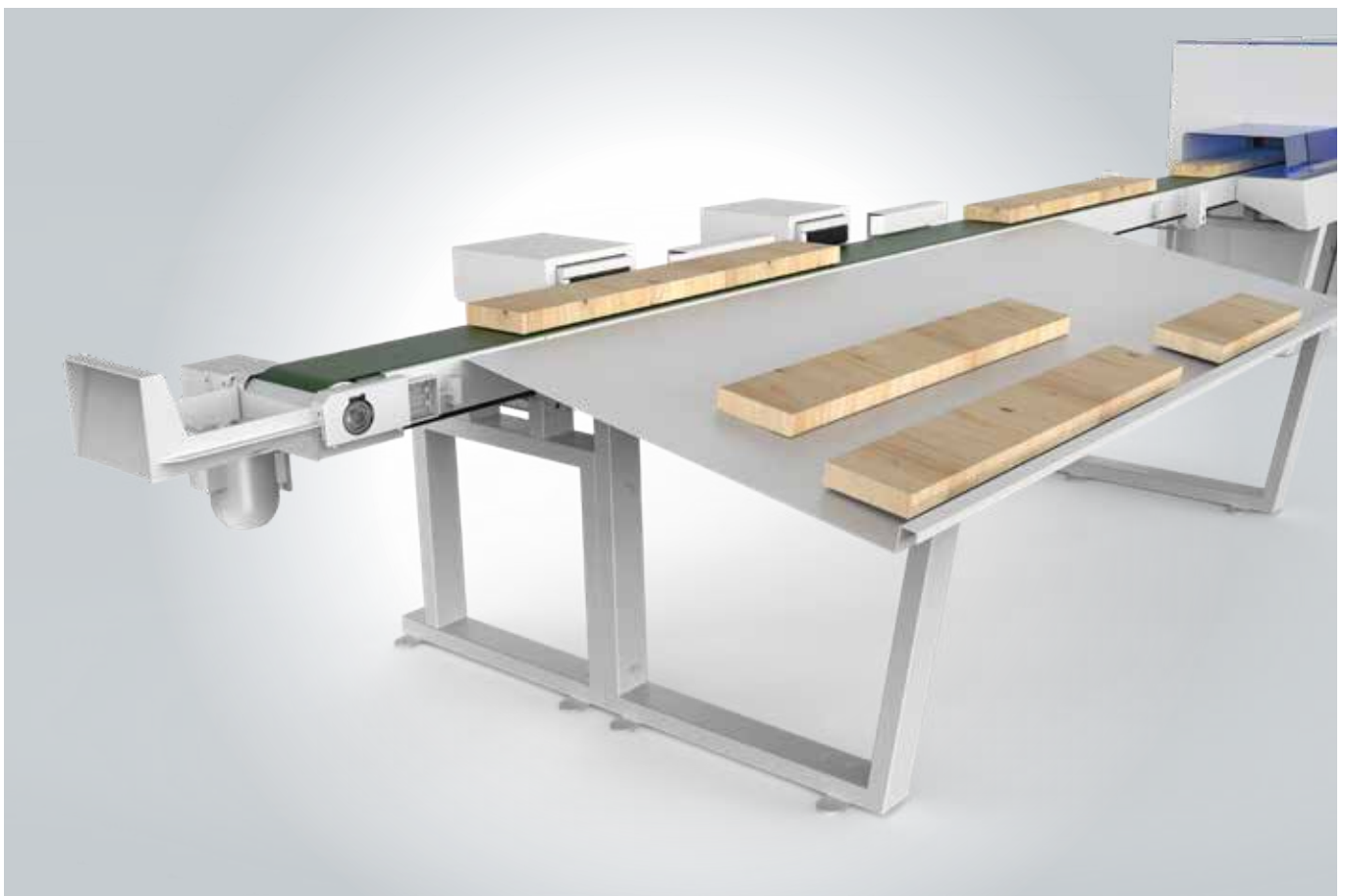
Automatic sorting system with kickers, available in different lengths and configurations, based on the different needs. The handling of the sorting system is integrated within the optimization software.
