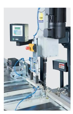
During the drilling process the workpiece is clamped pneumatically and directly below the drill spindle.
