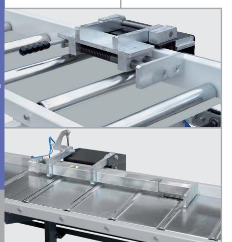
The stop is sprung mounted and can be folded backwards if necessary.
