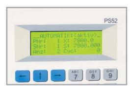
Up to 99 programmes with a maximum of 3,000 data sets can be saved in the control unit and recalled at any time at the push of a button.
