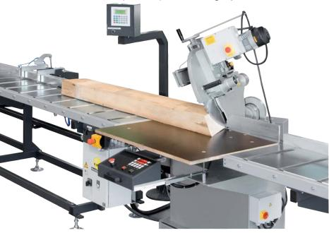
A programmable pusher or stop system is the core of the measuring system EXAKT NC.
