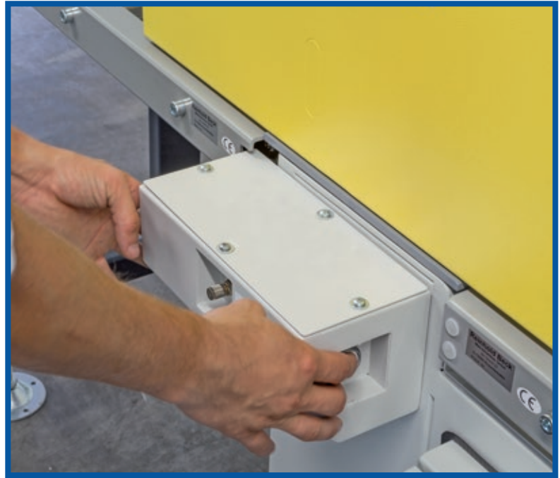
Operating elements The saw blade can be set into motion doubly secured must be operated with both hands. An adjusting screw regulates the saw blade feed.
