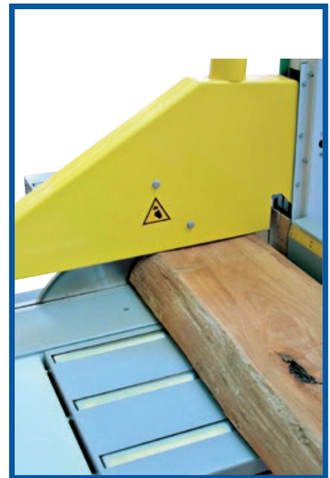
Blank holder The automatic blank holder holds the workpiece while sawing is in progress.
