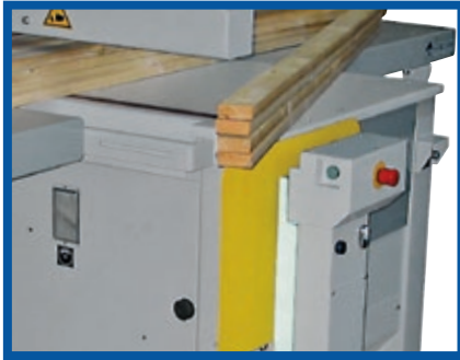
Safety shield can be lowered pneumatically (Option) Permits unhindered access to the workpiece. With integrated safety switch.
