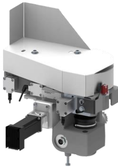
Pressure section DW501 MOT first roller driven, 2 support pressure rollers motorical with pneum. control of the pressure rollers PLC-controlled adjustment of edge thickness via NC servo-drive
