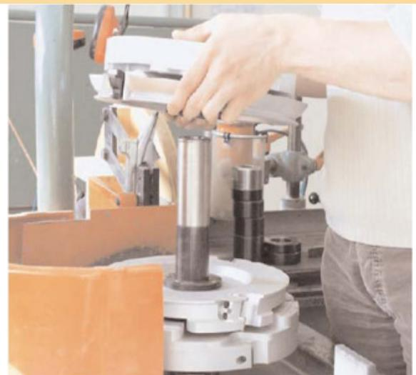
Leitz award winning RipTec System is used for planing, profiling and coping to improve finish and window performance while reducing scrap and tooling costs.
