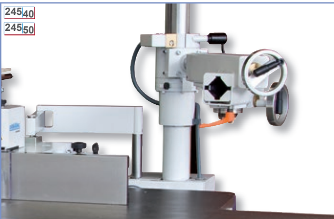
Comfort infed carrying arm, height-adjustable by electromotor, positioning via axis module for taking up a feeder item no.4216
