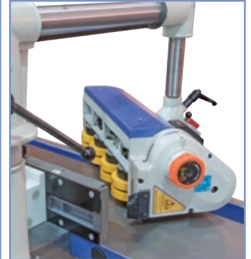
Infed device Variomatic 4N item no 4638 - 4 rollers (roller width separated 2 x 25 mm, rollers ø 120 mm) - Stepless speed 2 - 18 m/min - Right- and leftward operation - Quick change from horizontal to vertical operation - Simple tilting away and positioning - Memory-lock system for accurately repeatable fastening - Comfort stand - Numeric height display - Jib arm 1050 mm long
