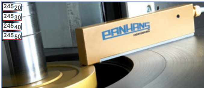
Zeromaster reference size setting device, ensures short setting up times in tool calibration
