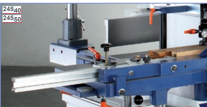
Sliding table item no. 4491 With stop holder, eccentric clamp, running track retractable, incl. safety hood 1641
