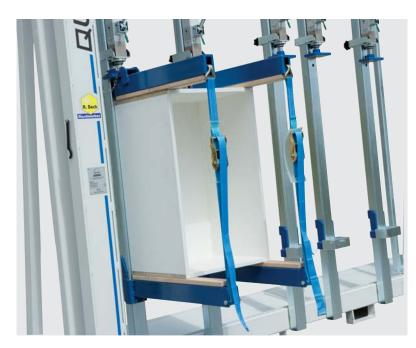
The manufacture of boxes become a walkover with the QUATTRA case press. The counter bearings and press element are simply fixed on the suitable vertical pressure beam and put into the right position. The press elements are supported by fine-adjustable belts for the rectangular pressing operation.
