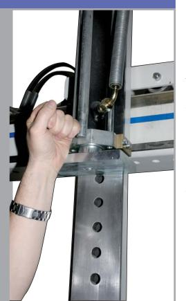
The hydraulic feeding system of HYDRO-Export is equipped with a variable pressure regulation of 30 - 150 bar and a manometer. An automatic pressure control with pressure downstream switching ensures pressure conservation which is operated through pushbuttons with separate control circuits for the vertical and horizontal jack cylinders.
