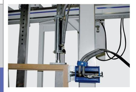
The moving carrier plate for width regulation can be adjusted through a central locking system in the 50 mm matrix of holes. HYDRO-Export disposes of two infinitely variable horizontal hydraulic jack cylinders with weight compensation for each jack cylinder. They have a double effect with 80 mm stroke and a press power of 30,000 N. The continuous left abutment for the width pressing operation is 80 mm deep.
