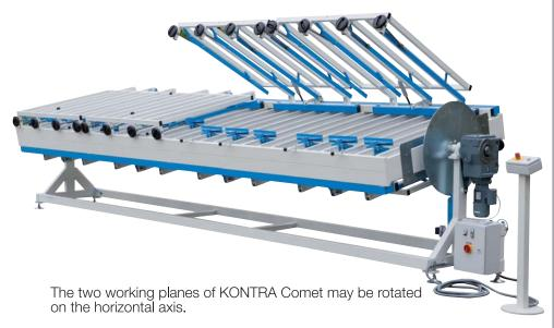
The rotary motion is carried out manually via a centrally fixed crank handle through a self-locking helical reducer or – by request – through an electrical driving motor.
