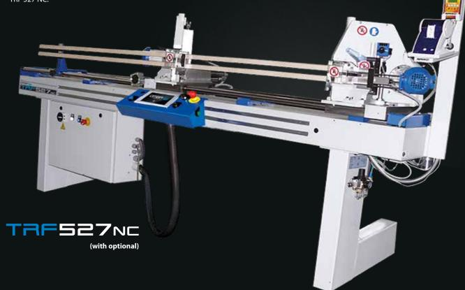
Mechanical stop for trimming to size. Allows frame glass stops to be trimmed without using a ruler.
