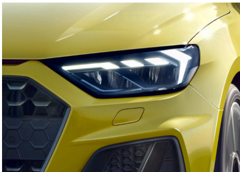
LED headlights with headlight washers
