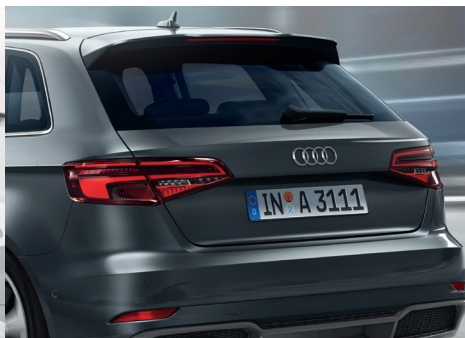
LED rear lights with dynamic indicators
