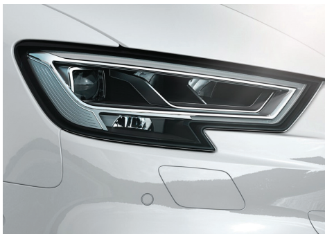
LED headlights with headlight washers
