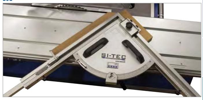
The DSG solves all tasks quickly and smoothly when producing mitre cuts on narrow and short workpieces at any angle from 0° - 90°.
