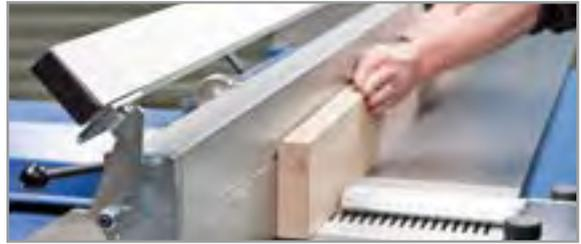
For secure surfacing of narrow work pieces at the surfacing fence.
