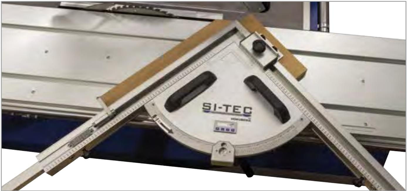
The DSG solves all tasks quickly and smoothly when producing mitre cuts on narrow and short workpieces at any angle from 0° - 90°.
