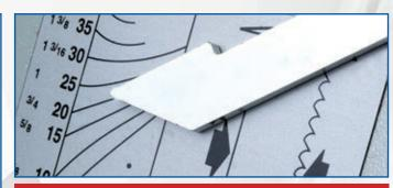
Blade tension display with sight window to set the recommended tension.
