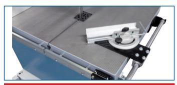
Mitre stop Top with round rod guide and device for folding away (retrofittable).
