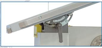
Table swivel facility with scale and clamping lever, smoothly adjustable up to 45°.
