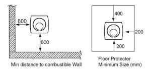
It is recommended that the fireplace be installed at least 800mm from combustible materials. However, any household furnishings should be at least 1000mm away as they could be adversely affected by heat.
