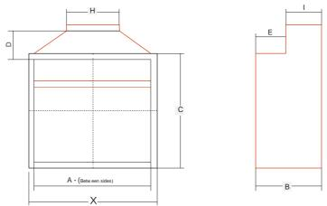
Please note: Dimension A is from the sides of the unit, to calculate the brickwork opening required. Dimension X is the overall width of the unit, measured from flat bar to flat bar.
