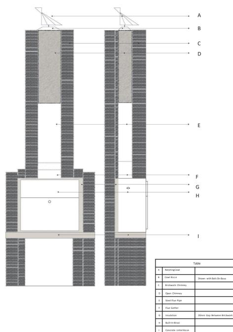
9 Fig. 1 Typical Installation of Megamaster unit.
