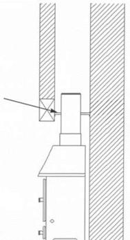
Fig 8: Horizontal register plate with top flue connection
