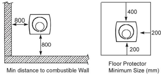
It is recommended that the fireplace be installed at least 800mm from combustible materials. However, any household furnishings should be at least 1000mm away as they could be adversely affected by heat.
