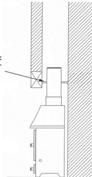
Fig 8: Horizontal register plate with top flue connection
