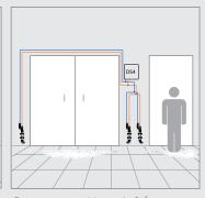
Foam pattern: Up to 6x3 ft. at each nozzle Spray tip: ST8060-1/2
