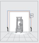
Foam pattern: Up to 8x4 ft. at each nozzle Spray tip: ST80100
