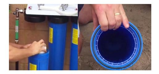
7. Ensure the cartridges center hole are seated in the stump in the base of each housing. Ensure the cartridge is centered & vertical as you lift the housing up into the head cap thread to replace. Hold 1 hand under the housing as you screw back on the
