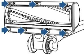
**2.** Remove the sole plate from the bottom of the foot by unscrewing the seven screws with a Phillips-head screw driver.
