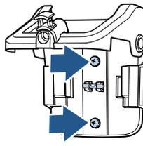
**2.** Insert two screws to secure to wall.
