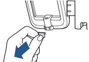
**3.** Insert the tool holder into the side of the Wall Storage & Charging Station. Remove the power cable clip.
