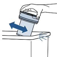
**3.** Fully remove the separator from the tank and tap the mesh screen on the side of the trash bin.
