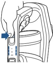
**1.** Press the Power Button to begin cleaning and to turn OFF the machine when finished cleaning.
