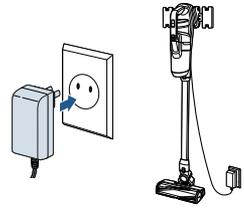
**6.** Plug the power adapter into the wall and place the machine on the station for charging. Refer to page 6, "Charging the Battery" for instructions.
