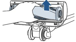
**3.** Pull the Brush Roll straight up and out of the chamber to remove.
