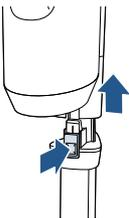
**1.** Press the release button to disconnect the Extension Wand.
