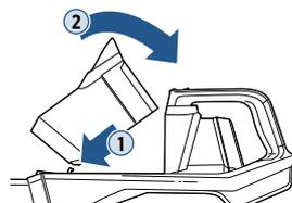
**6.** Put the whole tank into the hand vacuum by guiding the notched out area on the bottom of the tank onto the hook on the hand vacuum. Push into place.
