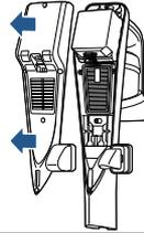
**3.** Pull the bottom cover off of the back of the machine.
