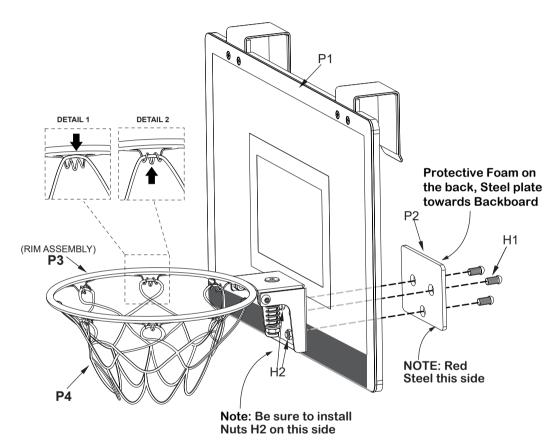
NOTE: After continued play, if Rim sags, slight tightening of the H5 Breakaway Rim Lock Nut may be required. Do not overtighten Nut as this would DEFEAT the breakaway function of the rim.
