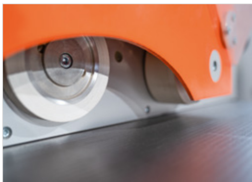
Circular saw feeder 76: Infeed roller in detail
