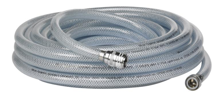
This hose is ideal for cleaning with water up to  $40^{\circ}$  C. It is equipped with a 1/2" Q-coupling in both hose ends. Water tap nipple, 0700 provided for 1/2", 3/4" and M22x1 screw thread types. Can be used with the following Vikan Q-couplings 0700, 0705 and 0712 as well as other Vikan products equipped with a 1/2" Q-nipple.
