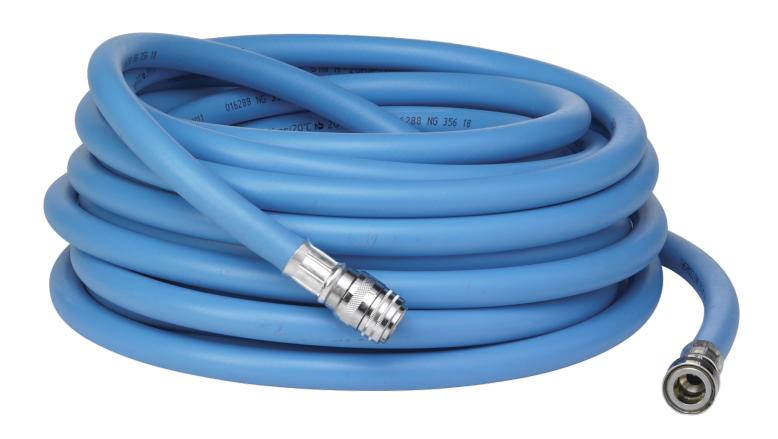
This Hot Water Hose is ideal for cleaning with water up to 70° C. It is equipped with a 1/2" Q-coupling in both hose ends. Water tap nipple, 0700 provided for 1/2", 3/4" and M22x1 screw thread types. Can be used with the following Vikan Q-couplings 0700, 0705 and 0712 as well as other Vikan products equipped with a 1/2" Q-nipple.
