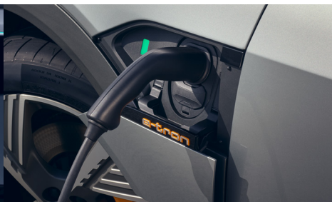
Fast charging with DC at up to 120kW and AC at up to 11kW
