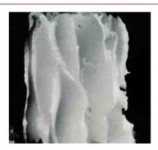
Substance processed with an EXAKT Classic 50 three roll mill shows a uniform and fine consistency of the substance.
