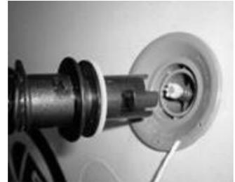
***NOTE: This inflation adaptor will automatically open the valve when inserted and will close the valve when removed. You do not need to manually open/close the valve when using this special adaptor.***
