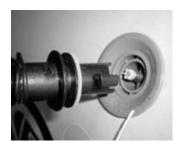
NOTE: This inflation adaptor will automatically open the valve when inserted and will close the valve when removed. You do not need to manually open/close the valve when using this special adaptor.
