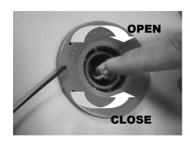
To lock open valve, depress stem and rotate ¼ turn clockwise. To close valve, depress stem and rotate ¼ turn counterclockwise. The valve stem should be in the depressed position while inflating. Replace cap on valve after inflation to ensure air tight seal.
