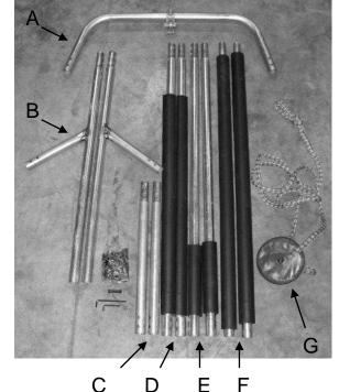
Insert frame pieces D into the other ends of C. Insert bolts and hand tighten. At this time, frame pieces A, B, C & D should all be laying flat on the ground.
