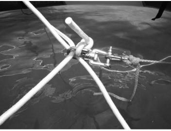
Remove all slack from anchor line and secure to swivel. Make sure the swivel is free to rotate. We recommend the (RAVE Anchor Connector Kit #01024).
