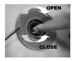
To lock open valve, depress the stem and rotate ¼ turn clockwise. To close valve, depress the stem and rotate ¼ turn counter-clockwise. The valve stem should be in the depressed position while inflating. Replace cap on valve after inflation to ensure air tight seal.
