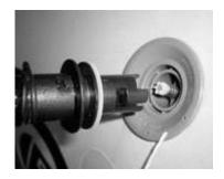
NOTE: RAVE Sports' special adaptor found on the High Speed Inflator and Digital Pressure Gauge will automatically open the valve when inserted and will close the valve when removed. This will ensure no air is lost when you remove the inflation nozzle. You do not need to manually open/close the valve when using this special adaptor.
